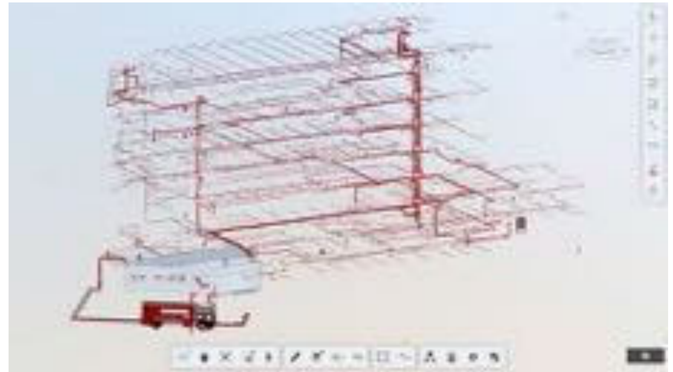
Fire Protection system In BIM Model
